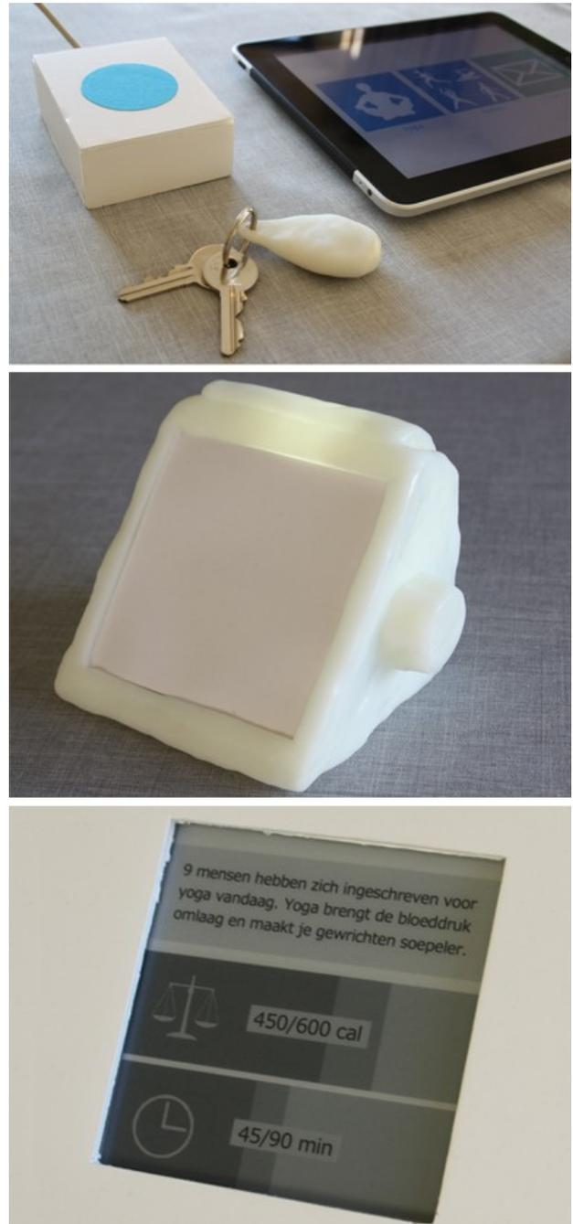
Figure 3: Message and tracking terminal with RFID-reader, keychain and iPad application (top). Physical glowing model of device in flat (middle). Representation of e-paper display for device in flat (bottom).
