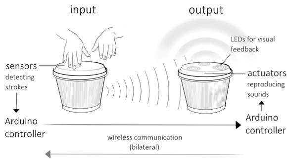
**Figure 2. Schematic representation of the Drum2Drum project.**
